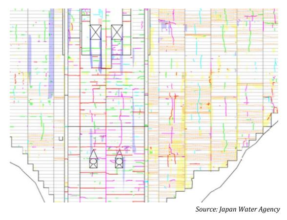
Figure 14 Sample of crack map
