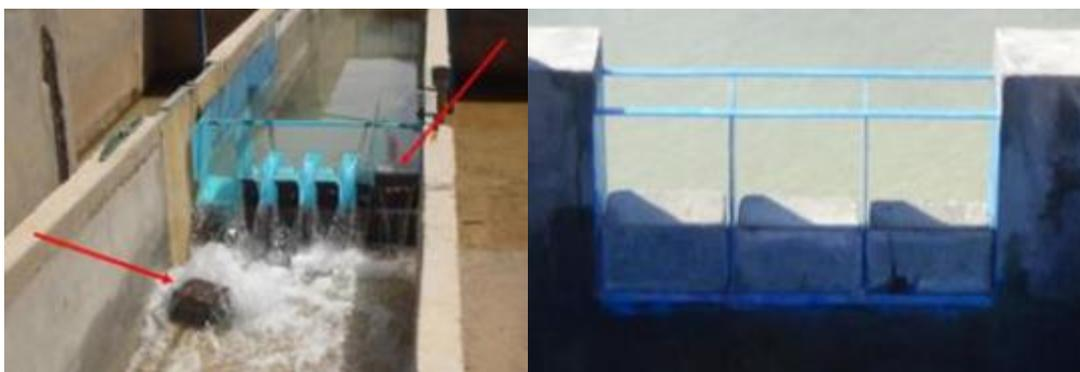
Figure 3-89: Physical model of concrete fuse plug alone and in combination with PK weir (University of Bistra).
