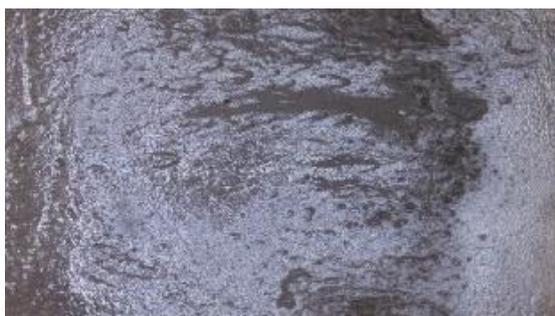
Figure 4-45: Concrete surface after abrasion test (Wang, 2019)
