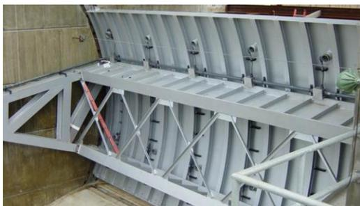
Figure 4-28: Tainter Gate at Spillway (Steel Fab Inc.)
