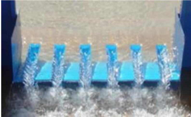
Figure 3-66: Typical physical model PKW's functioning (Epicum et al).
