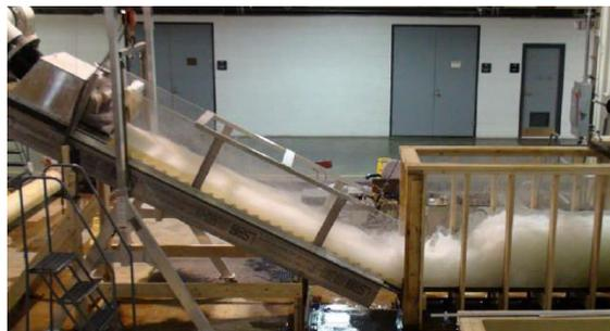
Figure 3-115: Hydraulic model stepped (slope 2:1), Stilling basin: USBR Type III (Frizell, et al.; 2016)
