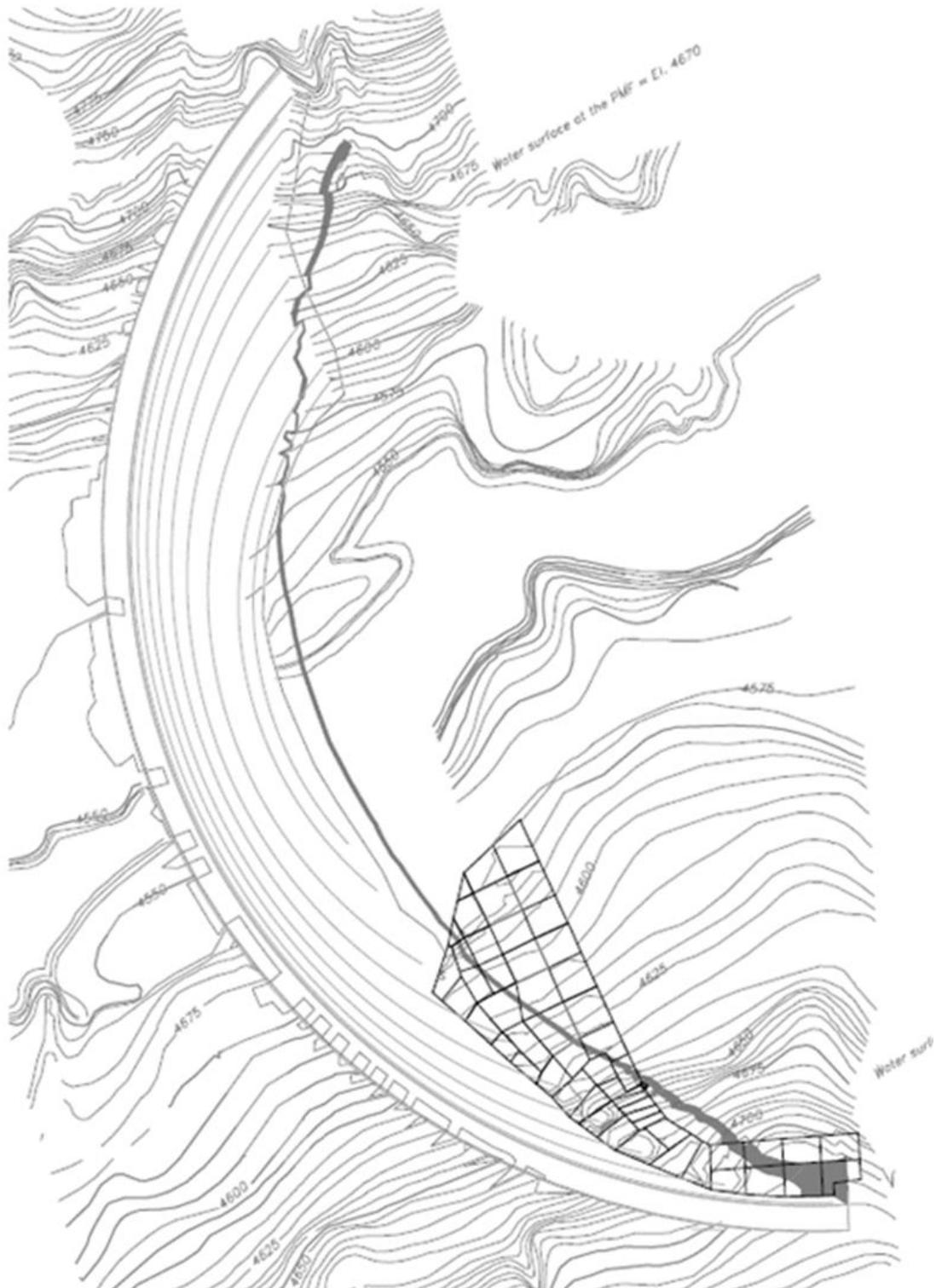
Figure 2-34: Footprint of the trajectory with no spread of the jet for the PMF overtopping at Gibson Dam
