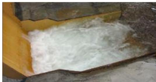
Figure 5-13: Typical model of stilling basin with drowned jump (FEMA, 2010)
