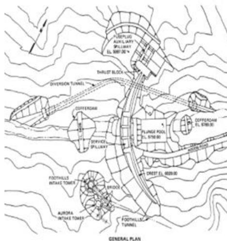
Figure 3-44: Strontia Springs Dam (South Plate river, Colorado, USA), fuse plug on left abutment. (Coleman and Wei).
