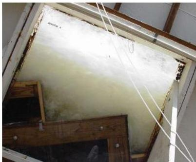
Figure 3-105: Skimming flow over 0.30 m high step with  $q = 1.4 \text{ m}^3/\text{s}/\text{m}$  (CSU, USBR)
