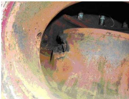
Figure 4-41: Globe Valve Cavitation damage (General Technical Knowledge; 2017)
