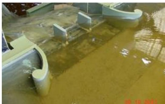
Figure 2-38: Approach channel and transition structures to connect with the ungated control structure, El Guapo Dam Spillway, Venezuela,. Scale Model 1:2, Edelca Hydraulics, Lab. (Photo A Marcano)
