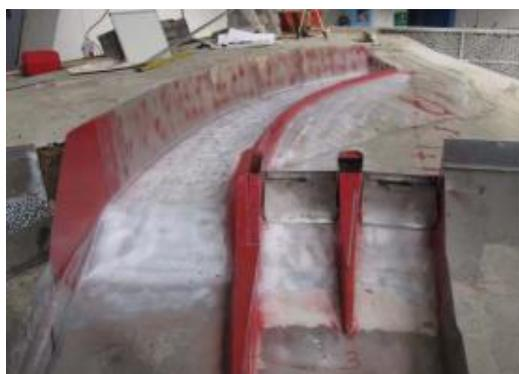
Figure 2-13: Front view of floating debris diversion structure
