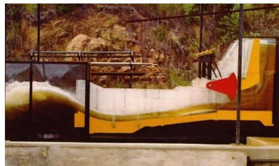
Figure 3-36: Breast spillway model Esc 1:27, as tested as an alternative of service spillways for Caruachi Dam, Venezuela,  $H=50\text{m}$ ,  $Q=30,000\text{ m}^3/\text{s}$  (EDELCA)
