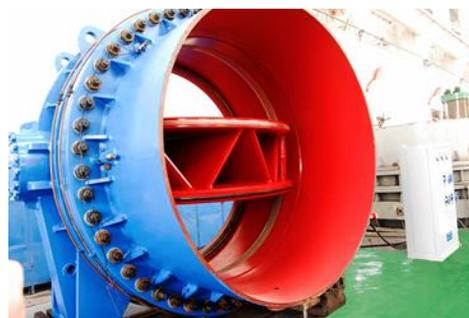
Figure 4-30: Butterfly Valve (FNencini SRL)
