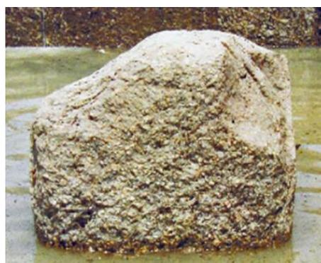
Figure 5-75: Concrete surface of a baffle block with cavitation's damages (FEMA, 2010)
