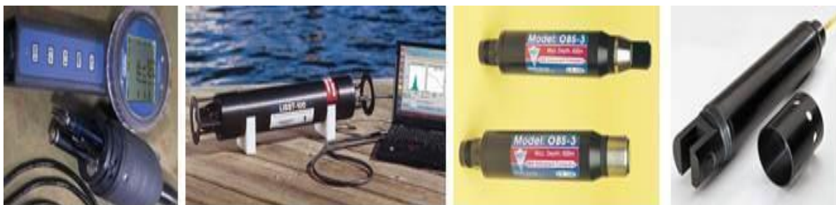
Figure D- 8 Images of Hydrolab Quanta water quality monitoring system, Sequoia LISST-100 sediment size distribution sensor, and D&A OBS-3 turbidity & suspended solid sensor; WQ710 turbidity sensor.
