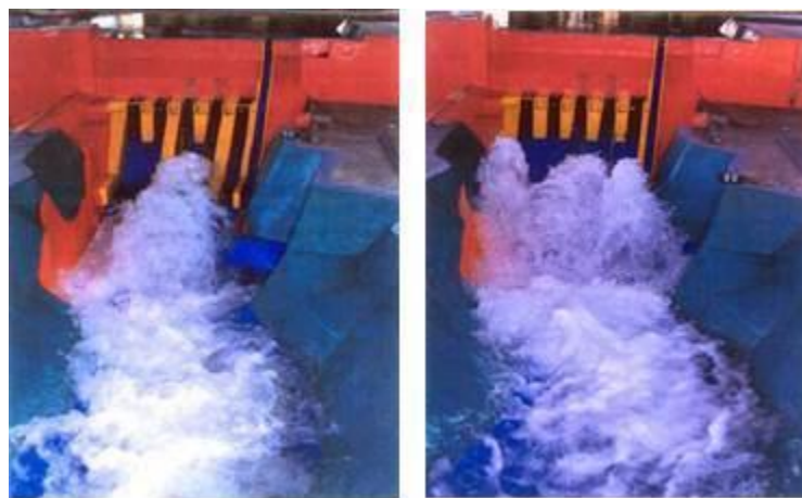
Figure D- 12 Model tests showing flow conditions downstream of spillway with (left) and without (right) divide walls.
