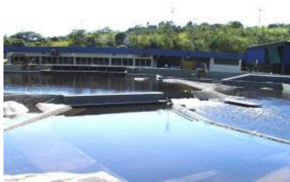
Figure B.1- 82 Caruachi Hydroelectric Project –Comprehensive 3D Physical Model Scale 1.80. Frontal view. (Marcano, 2002)
