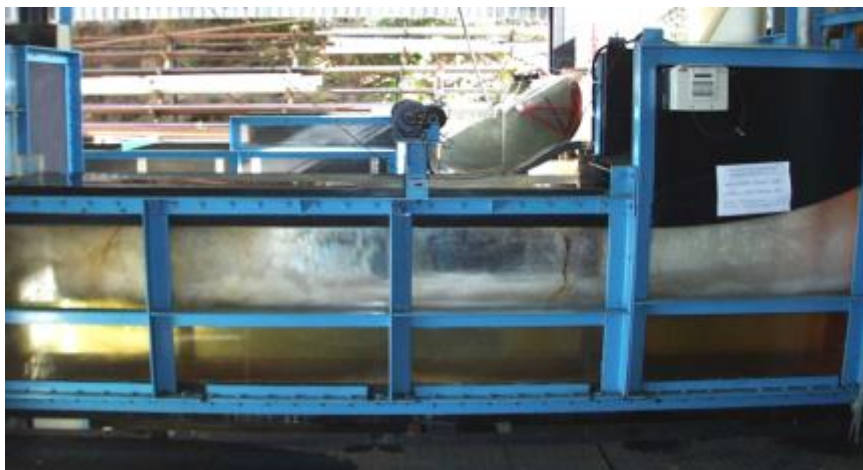
Figure B.1- 85 Caruachi Hydroelectric Project. Sluice and gate model Esc 1:13 to study down pull forces during Sluice Emergency Closure. (Marcano, 2002)
