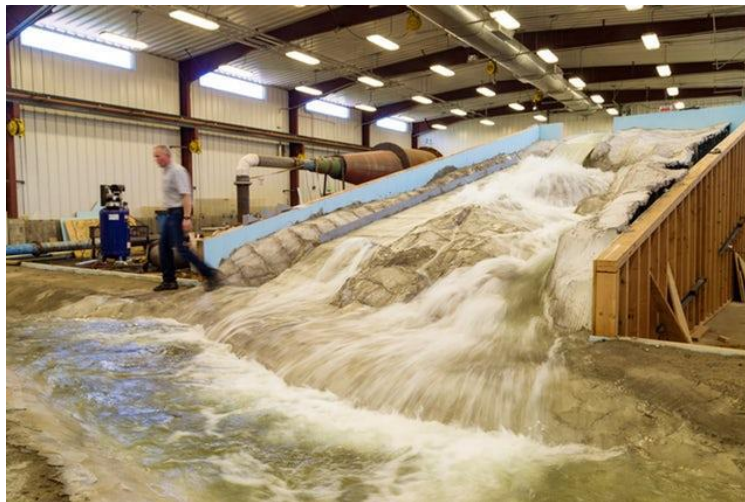
Figure D- 10 The 1:50 scale model of the damaged Oroville Dam spillway.
