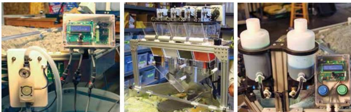
Figure D- 131(a) Groundwater control system; (b) Media feeder; and (c) Dye injector.
